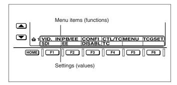
In the figure above, SDI (HD Serial Digital Interface signal) is selected as the setting for VID.IN (input video signal selection), the menu item for button F1. This manual refers to this as "F1 (VID.IN) in function menu HOME page is set to SDI."
