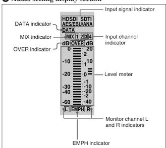
**Input signal indicator:** Indicates the currently selected input signal (HDSDI, SDTI, AES/EBU, or ANA for analog) for the corresponding audio input channel.
