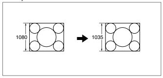
1080 ⇒ 1035 (CROP): Convert the active scan lines from 1080 to 1035. Crop the top, bottom, left, and right, then stretch the image horizontally.
