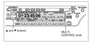
When the menu item number displayed in the menu display is flashing, you can change the menu item by turning the MULTI CONTROL knob.
