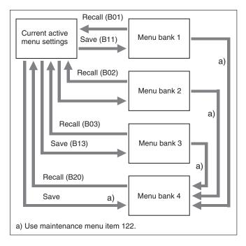
The current active setup menu settings as well as settings saved in menu banks are stored in separate storage areas for 59.94i, 29.97PsF, 23.98PsF and 50i, 25PsF, 24PsF modes.
